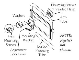
FIGURE 5.9 Repositioning the Joystick
